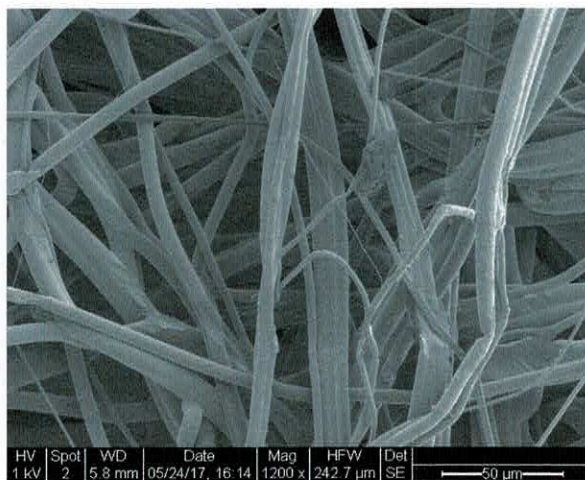
Figure 1. Scanning electron microscopy (SEM) image of meltblown microfiber fabric.
