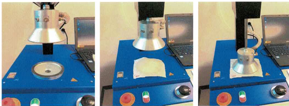
Figure 5. TSI 8130A for filtration efficiency and pressure drop measurement.
